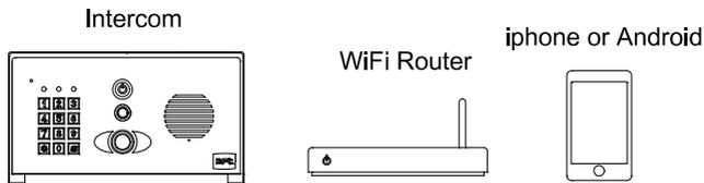
Locate the intercom on a bench or table beside the home router, along with the user phone. Connect the antenna & power supply provided to the intercom, red to +24v dc and black to 0v dc, and power on.
